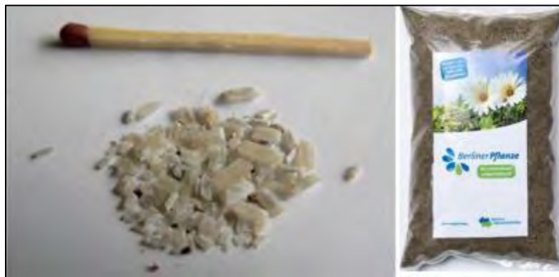
Figure 4. Struvite produced in AirPrex reactor, and packaged struvite fertilizer product
