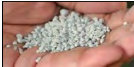
Figure 5. Struvite produced by PHOSPAQ reactor
