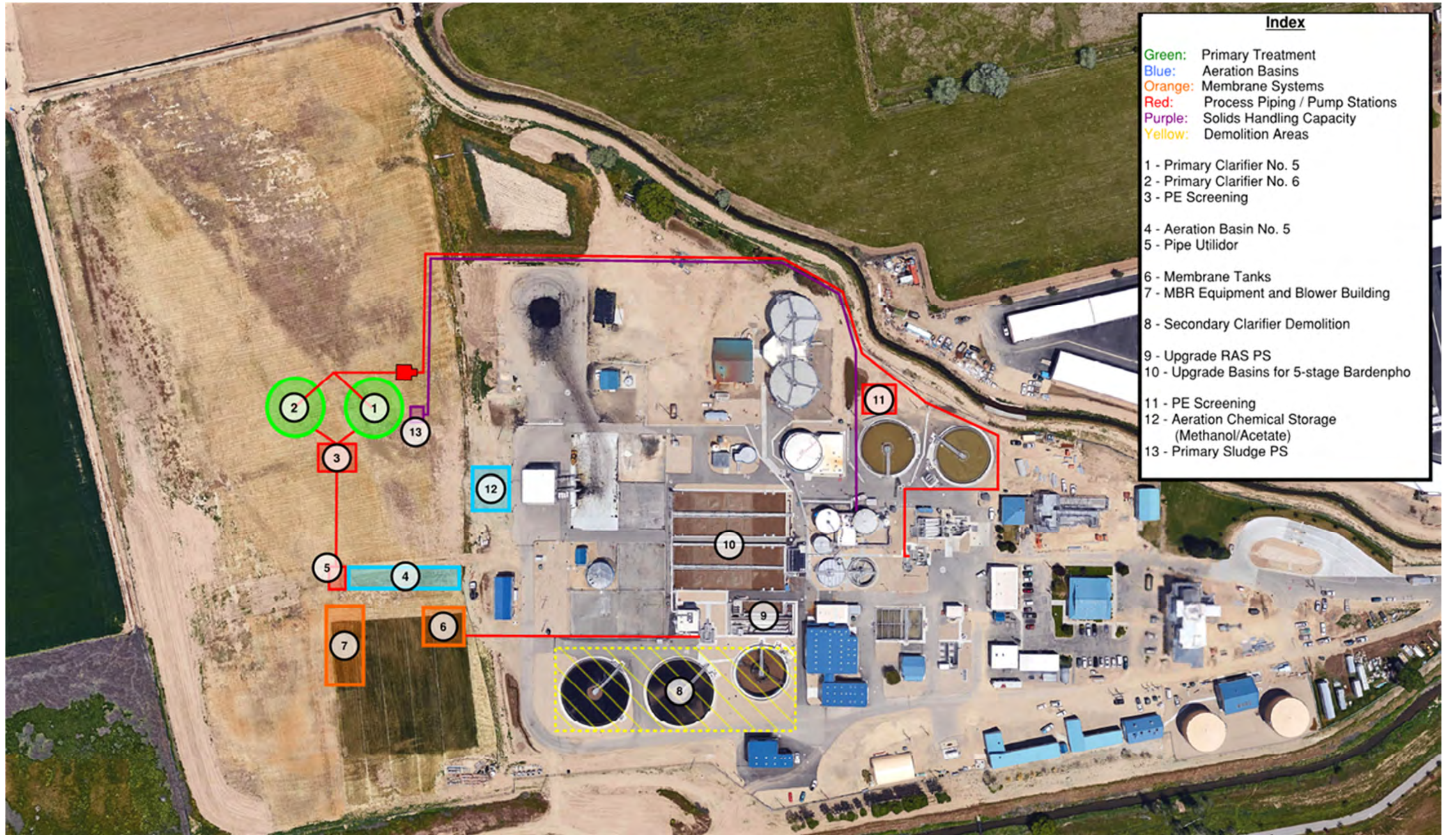
Figure 4-3. Plant layout for 5-stage Bardenpho with MBR
