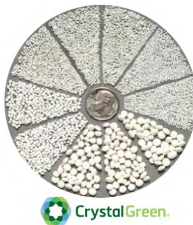
Figure 2. Struvite produced in a Pearl reactor 0.9, 1.5, 3.0, and 4.5 mm prill size (Source: Ostara)
